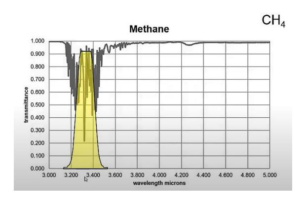
Every gas has a specific absorption wavelength in the IR band of the EM spectra
